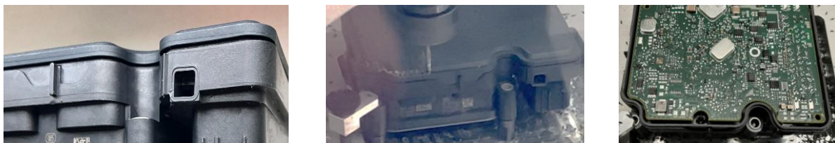
Figure 8: Destructive disassembly of laser welded plastic junction between housing and cover.
