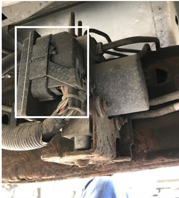
Figure 10 Rough environment for a BOSCH ESP at the underbody of a vehicle.
