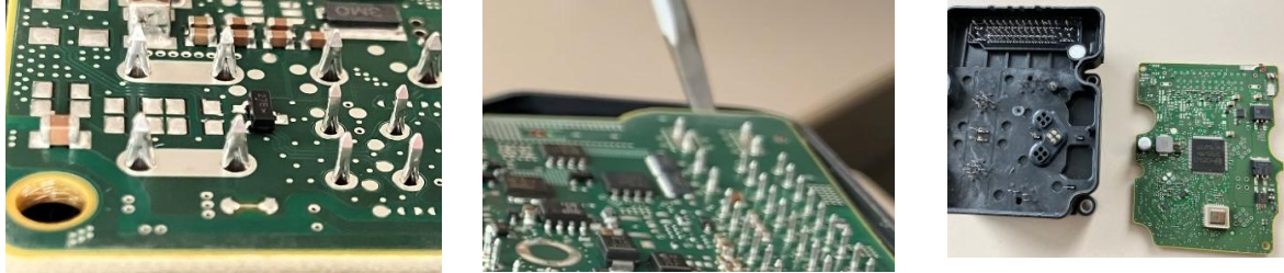
Figure 9: Destructive disassembly of press fit junction between PCB and Housing.
