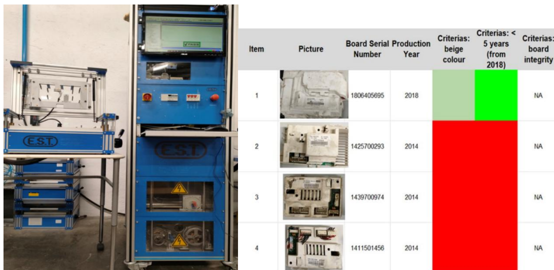
Figure 29: ATE test equipment and test results report extraction.
